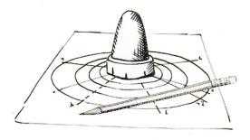
Use this tool to divide a circle into uniform parts. Center the work on the target below and make marks at the selected intervals.
